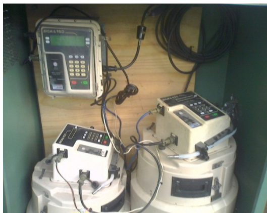
Figure 11. An example of the autosamplers used for wet weather water quality sampling. Two samplers were required for the samples analysed.
