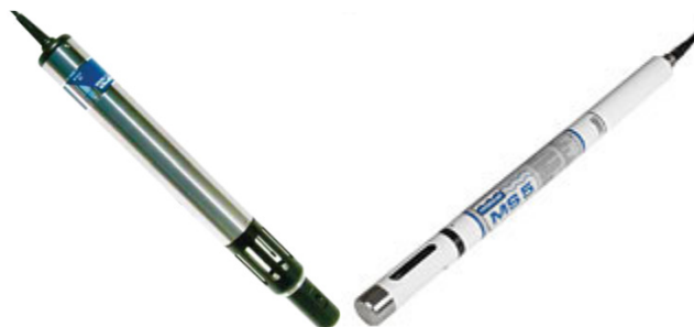
Figure 10. Water quality probes used in this study: the Greenspan CS304 (left) and the Hydrolab MS5 (right).
