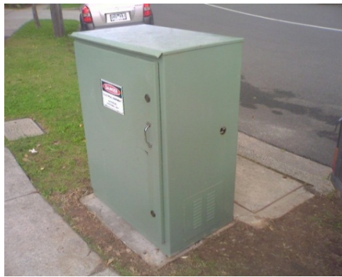
Figure 8. An example of the monitoring huts located at the Hedgeley Dene and Nunawading sites. These huts contained the autosampling equipment required to conduct wet weather sampling at these sites.
